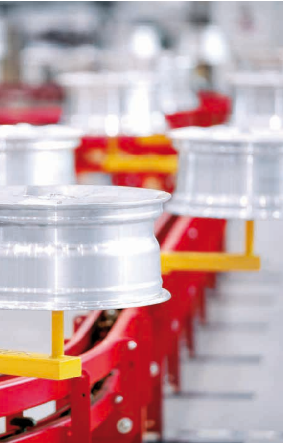
Inverted Power & Free conveyor for painting wheels.
