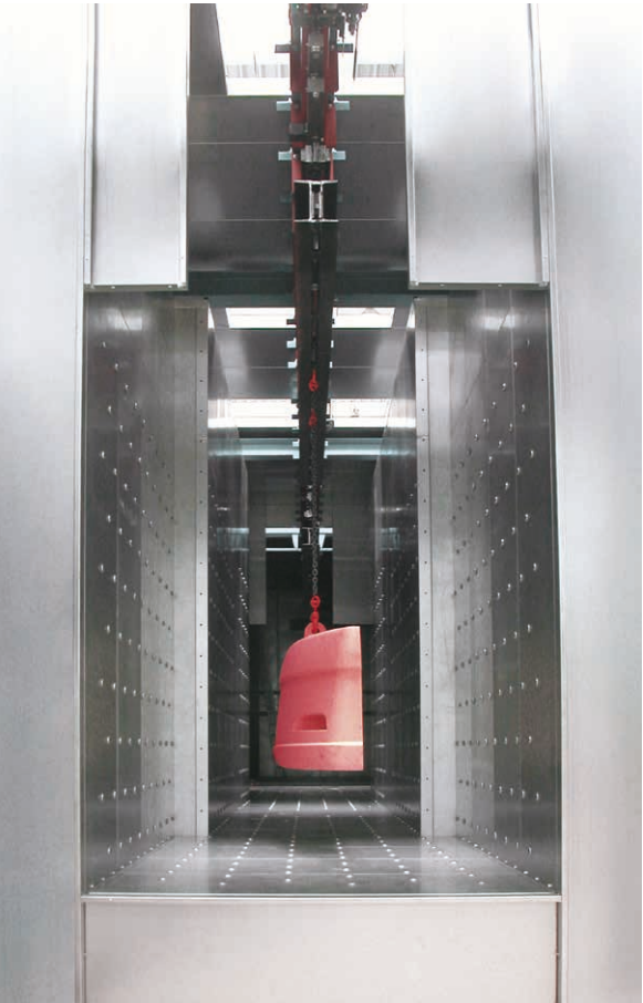
Power & Free for heavy loads in paint shops.
