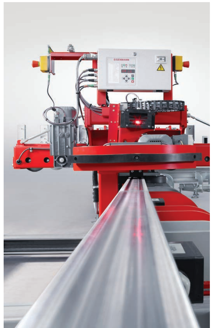
Inverted electrified monorail system with integrated roller conveyor.
