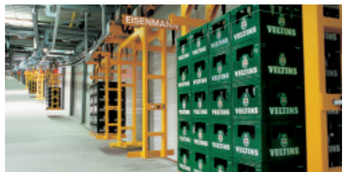
Gentle transport of sensitive goods to be transported even for gradients up to 45°
