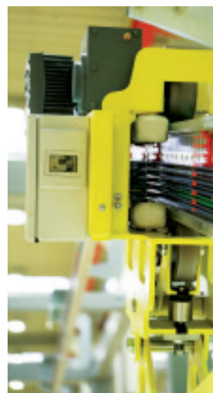
Eisenmann individual trolley with drives up to 3 kW.
