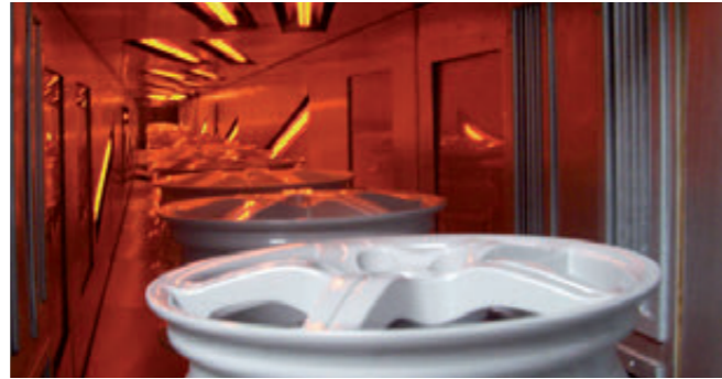
Infrared oven for preheating.
