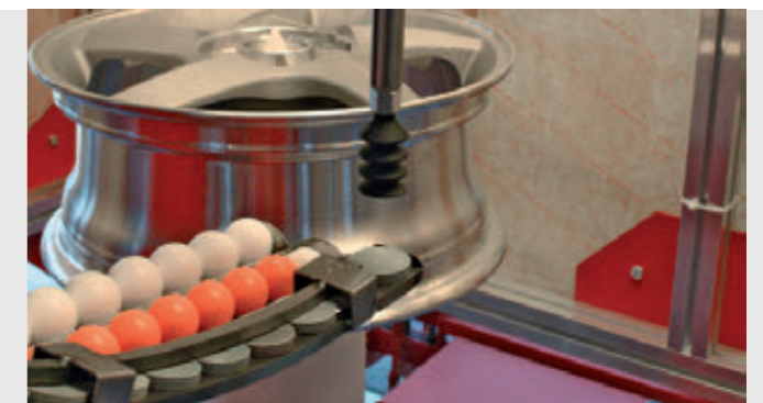
Automated masking of bolt holes with balls or taps.
