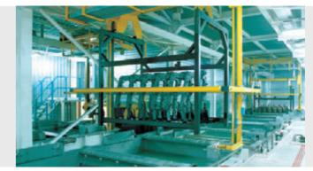
Electrophoretic dip coating is supremely suited to prevent corrosion, and can be used in mass production as well as for single-size lots.
