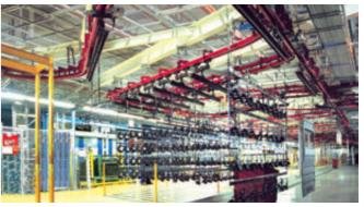
Complex power & free conveyor system with numerous pick-up stations, interim storage and process destinations in the automotive industry.
